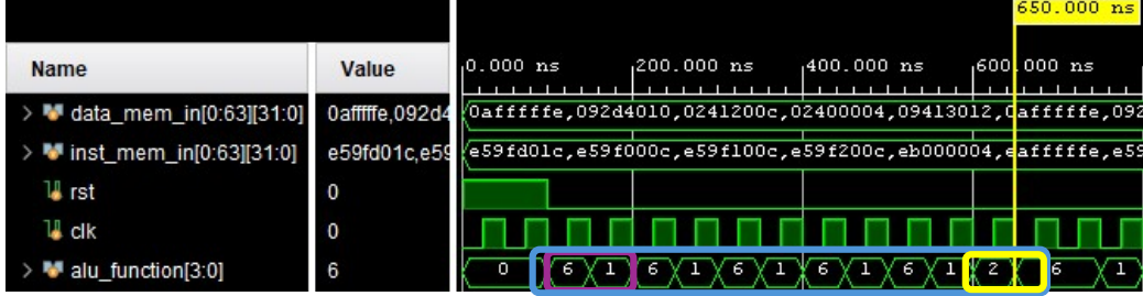
Figure 8.6: Simulation of the alu_func register during the execution of a neuron in the first hidden layer (blue: execution window of a neuron, purple: execution of multiplication and summation per connected input, yellow: execution of the ReLU function).
