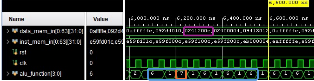
Figure 8.8: Simulation of the alu_func register during the computation of a neuron in the last layer after fault injection (blue: execution window of a neuron, purple: altered data register due to fault injection, orange: value of alu_func after fault injection).
